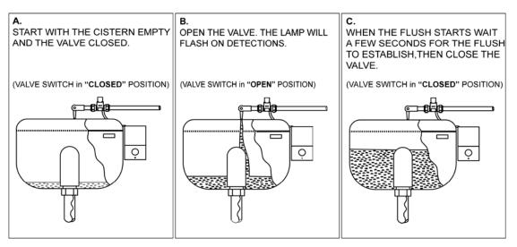
THE TIME TAKEN FOR THE CISTERN TO FILL IS STORED IN MEMORY AND USED ON ALL SUBSEQUENT AUTOMATIC FLUSHES.
